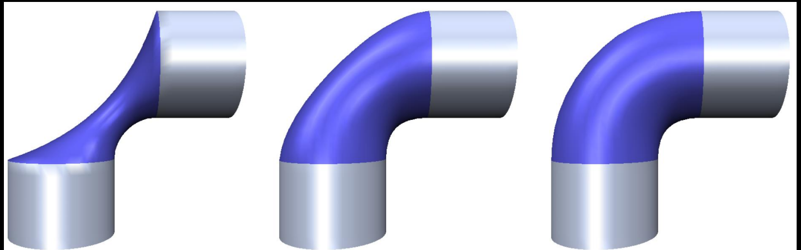
Figure 4.8. The blue region is determined by minimizing a fairness functional: membrane surface ( \Delta\mathbf{x} = 0 , left), thin-plate surface ( \Delta^2\mathbf{x} = 0 , center), and minimum variation surface ( \Delta^3\mathbf{x} = 0 , right). The order k of the Euler-Lagrange equation \Delta^k\mathbf{x} = 0 determines the maximum smoothness C^{k-1} at the boundary. (Image taken from [Botsch and Kobbelt 04a]. ©2004 ACM, Inc. Included here by permission.)
